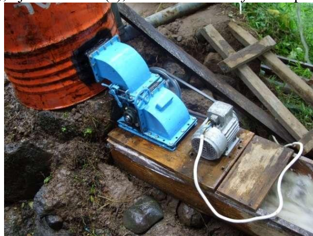
Gambar 9. Proses fabrikasi turbin Cross-flow : elbow (a), katup-nozel (b), tutup turbin (c), runner (d), uji keserasian (e), dan turbin Cross-flow siap dipasang (f)
